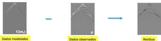
Figure: To search the right velocity model the difference of the synthetic en real seismograms is minimized
